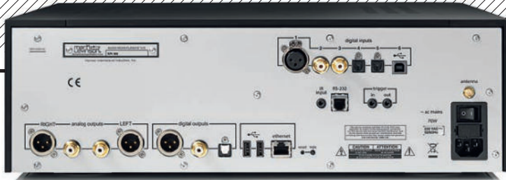
ABOVE: Two coaxial/optical S/PDIF digital ins are joined by USB 2.0 and AES/EBU ins, two USB-A sockets and wired/wireless Ethernet. Coaxial/optical and AES digital outputs are included alongside single-ended (RCA) and balanced (XLR) analogue outs
