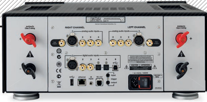
ABOVE: Two coaxial and optical S/PDIF digital ins plus USB and AES/EBU are joined by three RCA analogue line ins (one pre out), one balanced XLR in and 'Hurricane' 4mm speaker terminals. System controls include Ethernet, RS232, IR and 12V triggers
