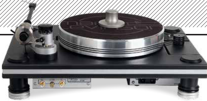
ABOVE: ML's triple-belt drive system is clear to see as is a variant of VPI's JMW tonearm base with its adjustable VTA tower. RCA sockets allow your choice of cabling
